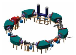
Figure 1 Schemmatic view of new ion cooler ring, S-LSR
