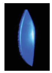
Figure 1. Cathode luminescence of SrTiO<sub>3</sub>.
