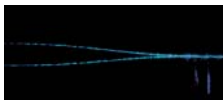
Y-branch channel waveguide directly written by UV laser irradiation. \text{Ar}^+ laser light (488nm) is coupled.
