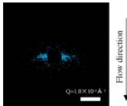
Fig. 1. 2D DPLS pattern of iPP at 1'57'' after shear.
