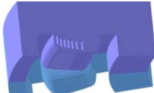
Figure 5. Configuration of the combined-function magnet. Its three dimensional magnetic field distribution is calculated with the computer code TOSCA.
