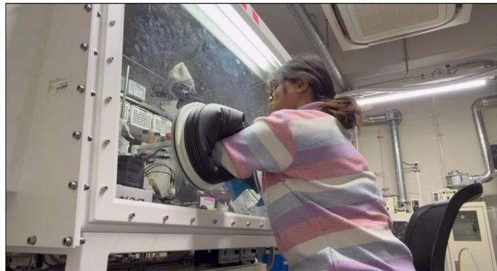
Figure 5: Working in the Glove box.
