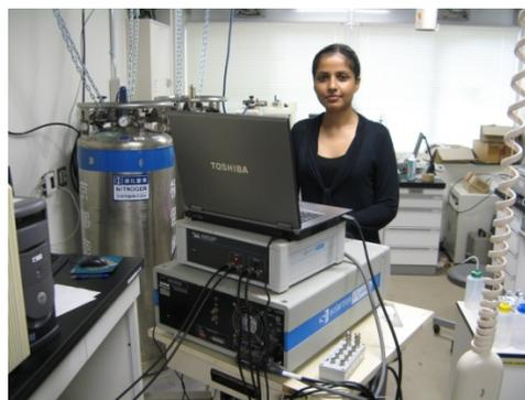
Operating rheo-dielectric set-up in the laboratory for studying the dynamics of entangled polyisoprene
