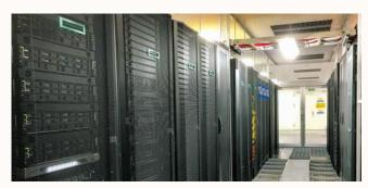
ICR Supercomputer System, equipped with HPE Superdome Flex (2×24 TB memory, 1,152 cores) and Apollo 2000 (5,680 cores), serves to accelerate researches in computational biology and chemistry.
