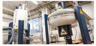
Dynamic Nuclear Polarization-enhanced NMR (DNP-NMR) System achieves great sensitivity enhancements. ICR also runs other solution/solid NMR machines including an 800 MHz one.
