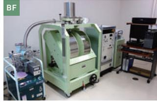
**振動試料型磁力計**
