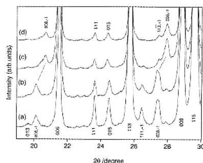
Partial enlargements of the XRD patterns of  $\text{Bi}_2\text{Sr}_x\text{CuO}_{6+\delta}$  as-prepared in  $\text{O}_2$  at 800°C (a), post-annealed in Ar at 200°C (b), 400°C (c), and 600°C (d).
