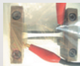
Ionic conductivity measurement with uniaxially stretched PEO.
