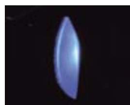
Fig.2 : Blue light emission from an oxygen-deficient \text{SrTiO}_3 single crystal.
