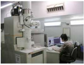
Figure 2. Cryogenic electron spectro-microscope: STEM/TEM, Field emission gun, Liquid He cryo-holder,  $\Omega$ -imaging filter, EELS,  $2k \times 2k$  CCD detector.
