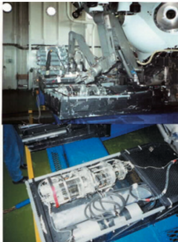
Figure 1. The in situ chemical analyzer GAMOS attached on the submersible "Shinkai 6500"
