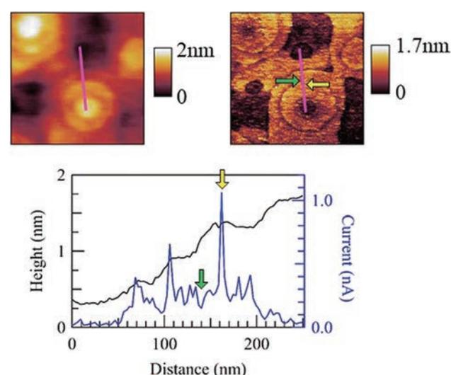
**Figure 2.** High-resolution topography and c-AFM images of the  $\text{SrFeO}_{2.5+\delta}$  film. In the bottom, cross-section profiles along the pink lines in the topography and conduction images are plotted.
