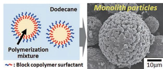
**Figure 2.** Preparation of epoxy resin-based monolithic particles.
