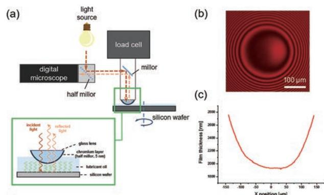
**Figure 1.** (a) Schematic diagram of an experimental set-up. (b) A photo image of the Newton's ring formed at the contact point. (c) A gap profile between a lens and a CPB-fabricated silicon substrate.
