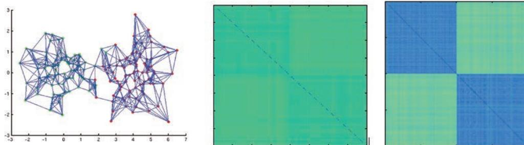
**Figure 1.** A graph (left) consists of two well-connected clusters. The distance based on graph Laplacian (heatmap in the middle heatmap) does not show cluster structure. Our new distance shows the two clusters by having two dark diagonal blocks on the heatmap (right).
