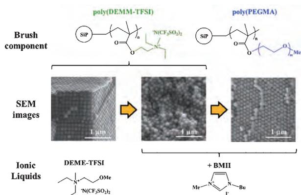
**Figure 1.** Cross-sectional SEM images of PSiP membranes obtained for different brush/ionic liquid components.
