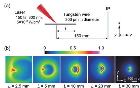
**Figure 4.** (a) Experimental setup for measurement of electron angular distribution. (b) Single-shot images detected by the IP. The color scale is set independently for each image for maximum contrast.
