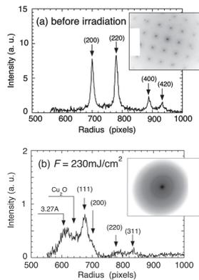
**Figure 1.** Electron diffraction patterns of thin Cu films (a) before irradiation and (b) at 0.23 J/cm<sup>2</sup>.
