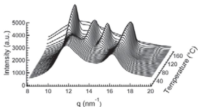
**Figure 1.** WAXD profiles during heating process from 30 to 170  $^{\circ}\text{C}$  displayed at every 5  $^{\circ}\text{C}$  from bottom to top. The profiles were shifted diagonally for clarification.
