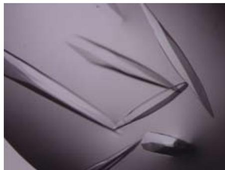
**Figure 1.** Crystals of psychrophilic MDH from *F. frigidimaris* KUC-1. The dimensions of the largest crystal were  $1.0 \times 0.15 \times 0.05 \text{ mm}$ .
