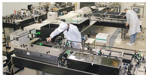
Ultra-intense femtosecond laser system for research of laser matter interaction science and collaboration in the Institute for Chemical Research (available from 2004 Autumn in the laser-building in the Advanced Research Center for Beam Science).
