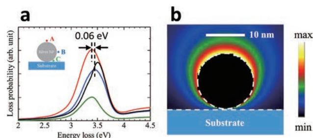
**Figure 2.** The EELS spectra and map calculated for a silver nano-sphere placed on an MgO substrate. (a) EELS spectra calculated for electron trajectories at the top, side and gap regions marked as A (red), B (blue) and C (green) in the inset, and that calculated for an isolated NP in a vacuum (black). These spectra were broadened by the instrumental energy resolution. (b) EELS map calculated at an energy of 3.40 eV.
