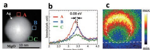
**Figure 1.** Experimental EELS results obtained from a silver NP placed on an MgO substrate, applying electron irradiation in the direction of the cross-section. (a) HAADF image, in which three 2 nm squares are indicated, each 1 nm from the NP surface. (b) EELS spectra obtained from the top, side and gap regions indicated in (a) as A (red), B (blue) and C (green). (c) EELS map generated using an energy window from 3.20 to 3.60 eV.
