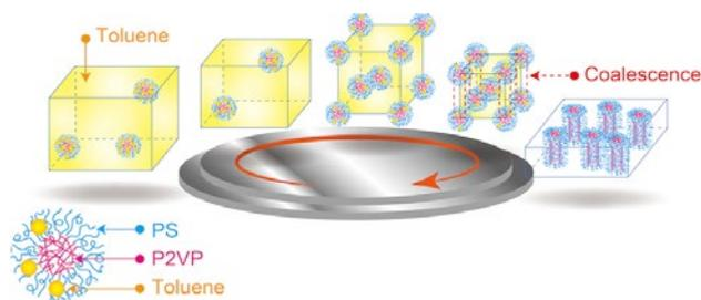
Figure 3. Spin-coating process of PS-P2VP thin film.
