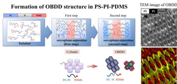
Figure 1. Formation of OBDD structure in PS-PI-PDMS.
