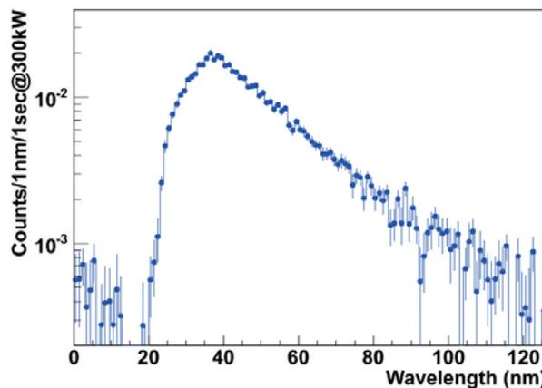
Figure 3. Result of the UCN transport experiment. We succeeded in measuring the UCN spectrum through the UCN guides of 5.6 m length.
