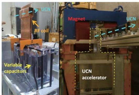
Figure 4. Photograph of the inner machinery of UCN accelerator (left) and experimental setup (right).
