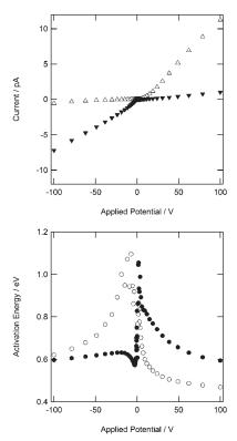
**Figure 1.** Variation in device current (upper) and the activation energy of electrical conductance (lower) as a function of applied potential, for the system after positive bias stress  $(\triangle, \bigcirc)$  and after negative bias  $(\mathbf{\nabla}, \mathbf{\bullet})$ .
