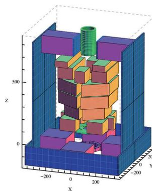
Figure 4. Permanent magnet focusing system designed with RADIA4.29.
