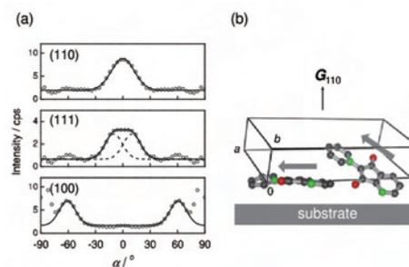
**Figure 2.** (a) X-ray pole figures (plotted as a function of polar angle  $\alpha$  measured from the surface normal) of (110), (111) and (100) diffractions for the 4*N*-PI film. (b) Schematic of the analyzed orientation of the unit cell with 4*N*-PI molecules on the substrate surface.
