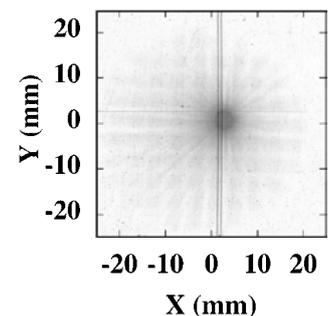
**Figure 3.** Radial distribution of the laser-produced proton beam after phase-rotation.
