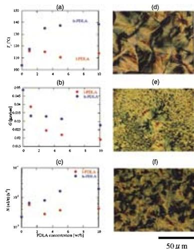
**Figure 1.** PDLA concentration dependence of crystallization temperature on non-isothermal crystallization (a), Growth rate (b) and Nucleation rate of PLLA spherulites on isothermal crystallization (c) (left) and OM final structure of PLLA (d), PLLA/l-PDLA3% (e) and PLLA/h-PDLA3% (f) after isothermal crystallization at 140°C (right).
