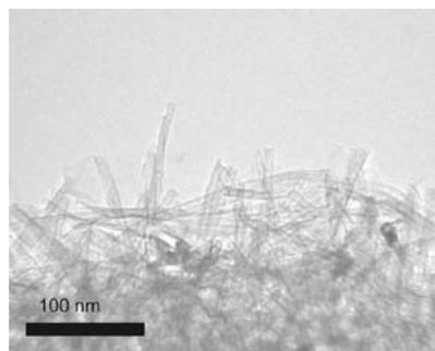
**Figure 1.** Typical TEM images of titanate nanotubes.
