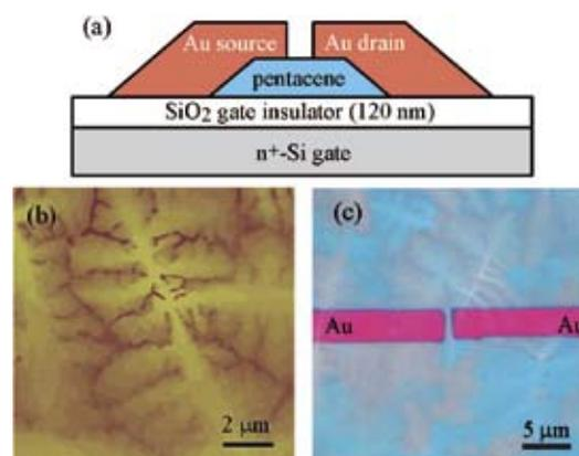
**Figure 3.** (a) Schematic cross section of a single-grain OFET with top-contact structure. (b) Morphology of vacuum-deposited pentacene film observed with an AFM. (c) Optical microscope image around a channel region of a single-grain OFET with  $1 \mu\text{m}$  of channel length.
