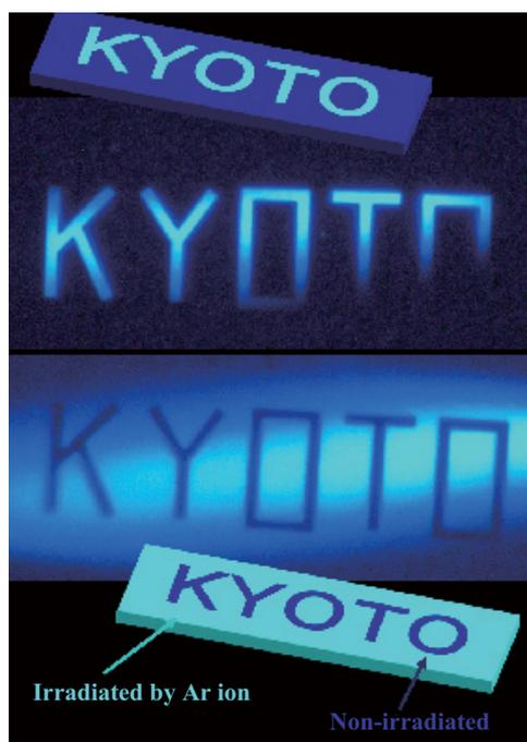
**Figure 1.** An example of the blue-light emission from a local engineered region of oxygen vacancies in SrTiO<sub>3</sub>.
