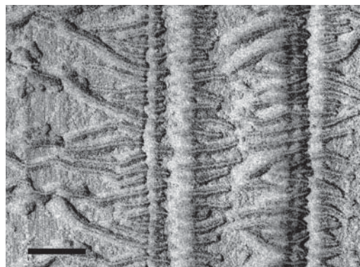
Figure 2. Nano-sized arrays prepared from atactic polystyrene. Scale bar is 500 nm. The molecular chains of PTFE are oriented vertically.
